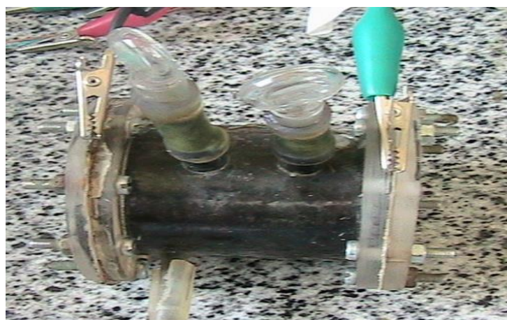
Figure 1: Membrane-less air cathode single chamber microbial fuel cell composed of anode and cathode electrodes connected with wire to close the circuit.
