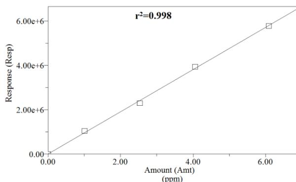
Fig (6): Gallium Standard calibration curve of the certified soil sample of the optimized developed method
