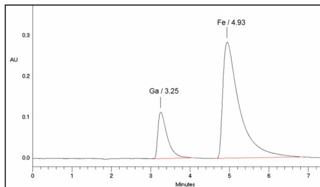
Fig (4): The chromatogram represented the separation of gallium and the nearest interfering iron
