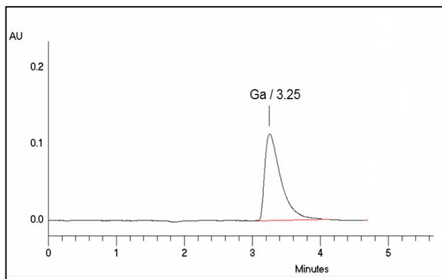
Fig (5): Separated gallium peak produced after injection of the certified soil sample (NCS DC 73325).
