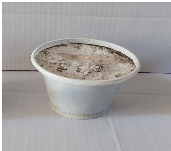
photo (1): fungus growth
