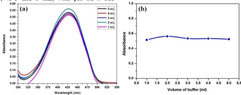
Fig (3): Absorption spectra of tartrazine (a) and the absorption value of tartrazine (b) using various volumes of universal buffer.
