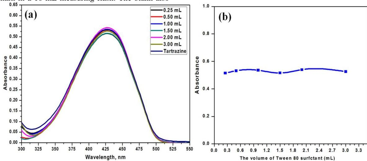
Fig (5): Absorption spectra of tartrazine without and with Tween 80 surfactant (a) and the effect of Tween 80 volumes on the absorbance values of tartrazine (b).
