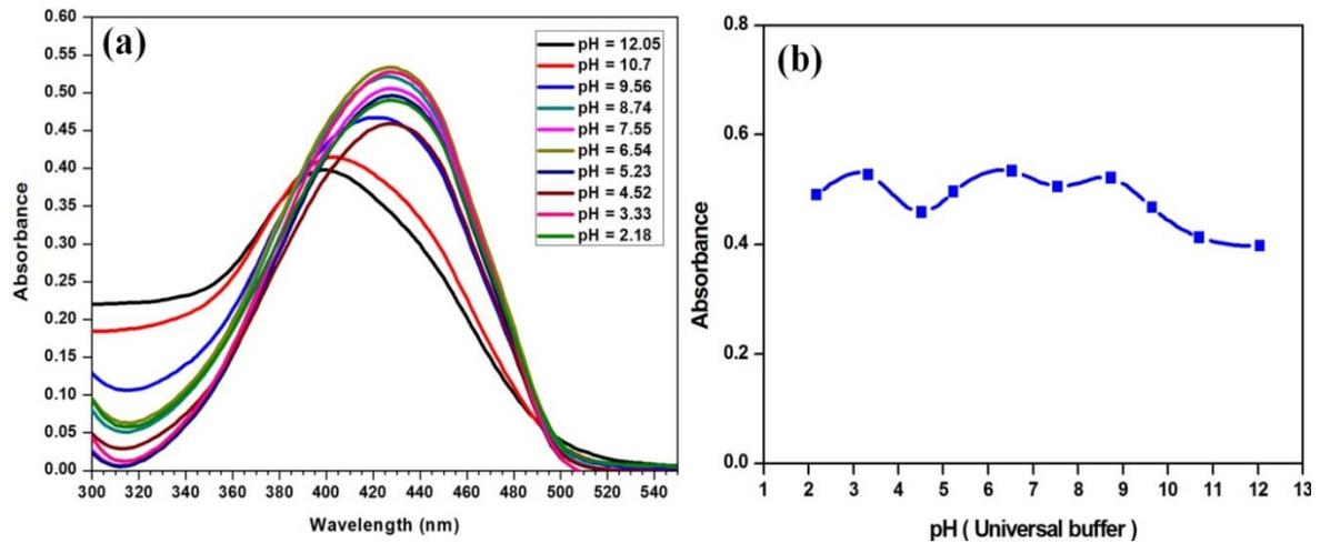
Fig (2): Absorption spectra of tartrazine at  $\lambda_{\max}= 427$  nm (a) and the absorption value of tartrazine (b) using a universal buffer with different pH [pH=2-12].
