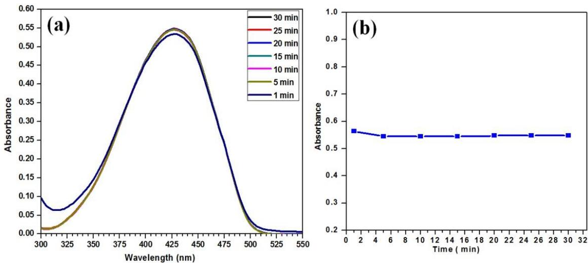
Fig (6): The effect of time on the absorption spectra (a) and the absorbance value with time (b) of tartrazine.
