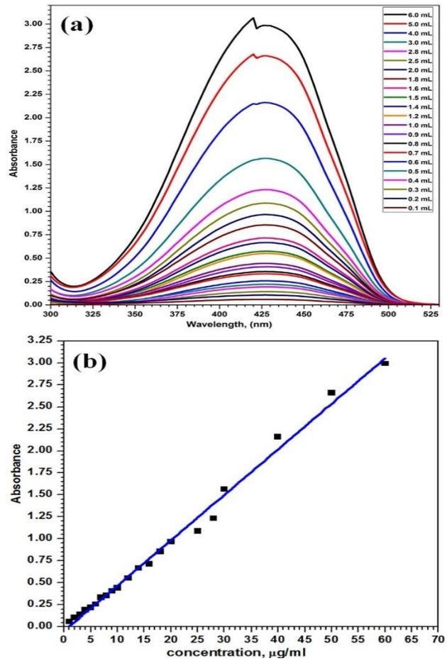
Fig (7): The absorption spectra of tartrazine with various concentrations (0.1 – 6 mL) and application of Beer's law for tartrazine using optimum conditions.
