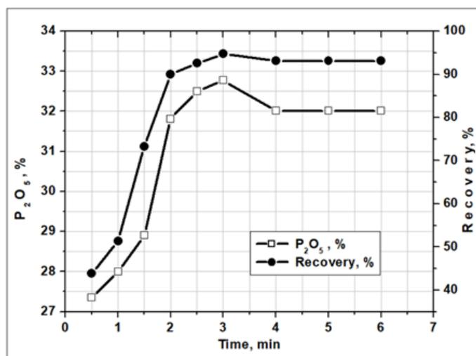
Fig (10): Effect of flotation time on the content; % and recovery % of apatite (100-75 μm particle size, 1.5 g/kg sesame oil collector, 6g/kg corn starch depressor, pH pulp 10 and 1:3 S/L ratio, 2000 RPM and 1.6 cm/s air superficial velocity) at 25°C.
