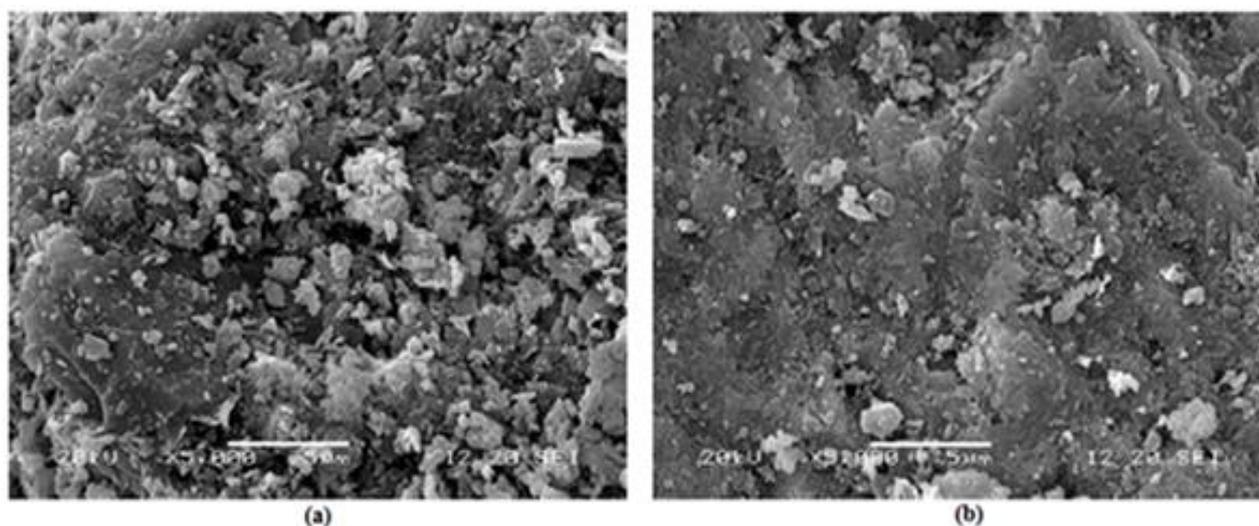
Fig (11): SEM of phosphate samples, (a) raw ore; (b) final concentration
