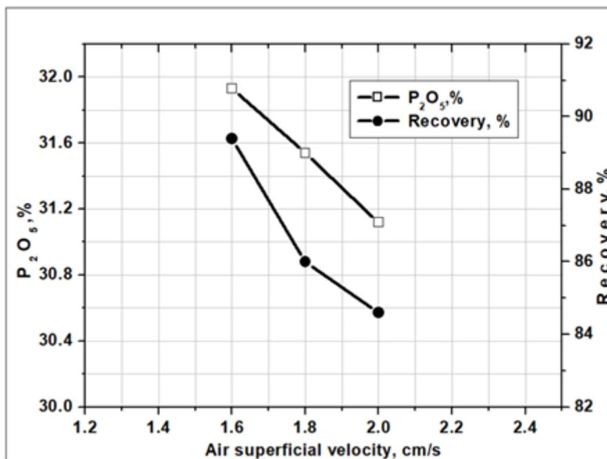
Fig (8): Effect of air superficial velocity on the content; % and recovery % of apatite (100-75 μm particle size, 1.5 g/kg sesame oil collector, 6g/kg corn starch depressor, pH pulp 10 and 1:3 S/L ratio, 2 min flotation time, 2000 RPM) at 25 °C.
