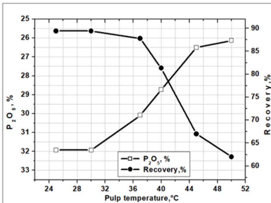
Fig. (9): Effect of the pulp temperature on the content; % and recovery % of apatite (100-75 μm particle size, 1.5 g/kg sesame oil collector, 6g/kg corn starch depressor, pH pulp 10 and 1:3 S/L ratio, 2 min flotation time, 2000 RPM) with 1.6 cm/s air superficial velocity.
