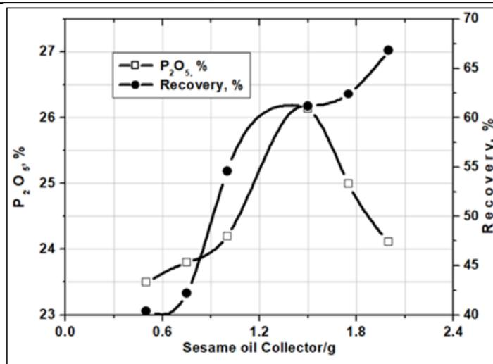
Fig (5): Effect of sesame oil soap dosage /g as a collector on the content;% and recovery; % of apatite (100-75 μm particle size, 2 g/kg corn starch depressor, 1:3 S/L ratio, pulp pH 8, 2 minutes flotation time and air superficial velocity 2.0 cm/s and 2000 RPM) at 25 °C.
