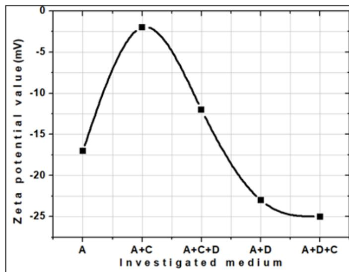
Fig (4): Zeta potential of apatite before and after mixing with collector and depressor at pH9
