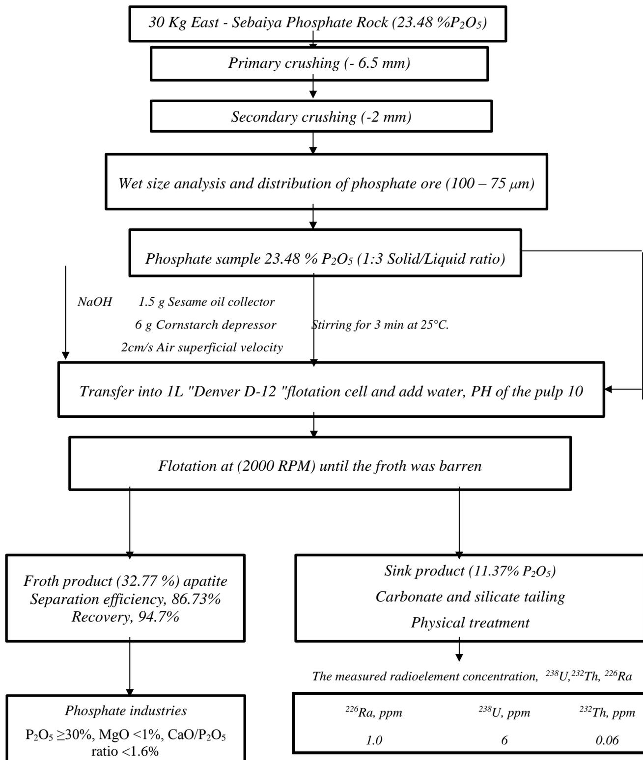
Fig (12): Flotation experiment circuit for the removal of silicate and carbonate.
