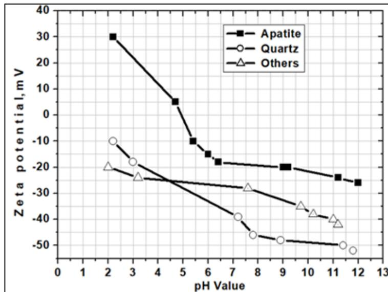
Fig (3): Zeta potential of apatite, quartz and clay dispersions as a function of pH
