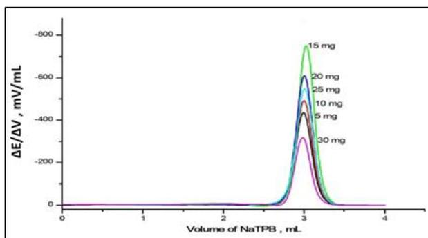
Fig (2): Effect of ALF-TPB content on the performance of CPEs in the potentiometric titration of 3mL of  $10^{-2}$  mol/L ALFHC with  $10^{-2}$  mol/L NaTPB.
