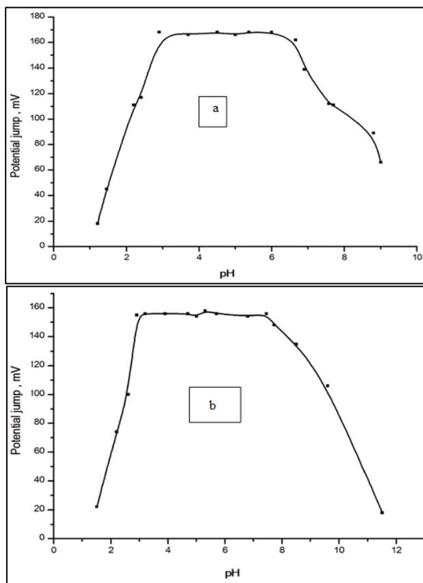
Fig (4): Effect of pH of the test solution on the performance characteristics of (a) electrode (I) and (b) electrode (II).
