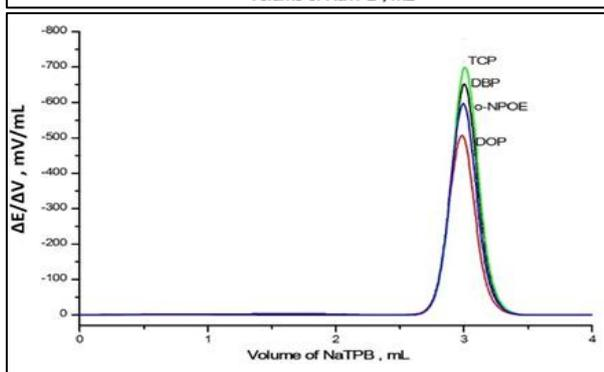
Fig. (3): The effect of plasticizer type on the MCPE performance in the potentiometric titration of 3 mL of  $10^{-2}$  mol L<sup>-1</sup> ALFHC with  $10^{-2}$  mol L<sup>-1</sup> NaTPB
